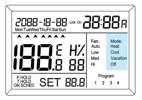
**Press MF 8 times, then OK for Heat mode.** Heat mode supplies hot air if the set temperature is greater than the room temperature.
