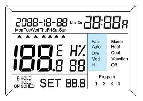
**Press MF 4 times, then OK for Auto.** The thermostat automatically sets the fan to High, Med or Low speed determined by the difference between room temperature and the temperature setpoint.
