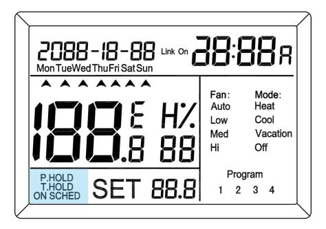
**Press MF once, then OK for P HOLD. P Hold or Permanent Hold** holds the selected settings and modes until otherwise changed. You'll be prompted to select a temperature setpoint using Up & Down.
