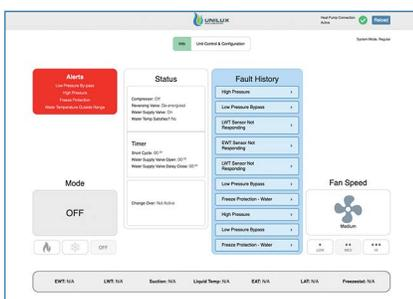
Fault history displays the 5 most recent alerts/faults. This section cannot be reset or overridden, so that all technicians can view previous faults.
